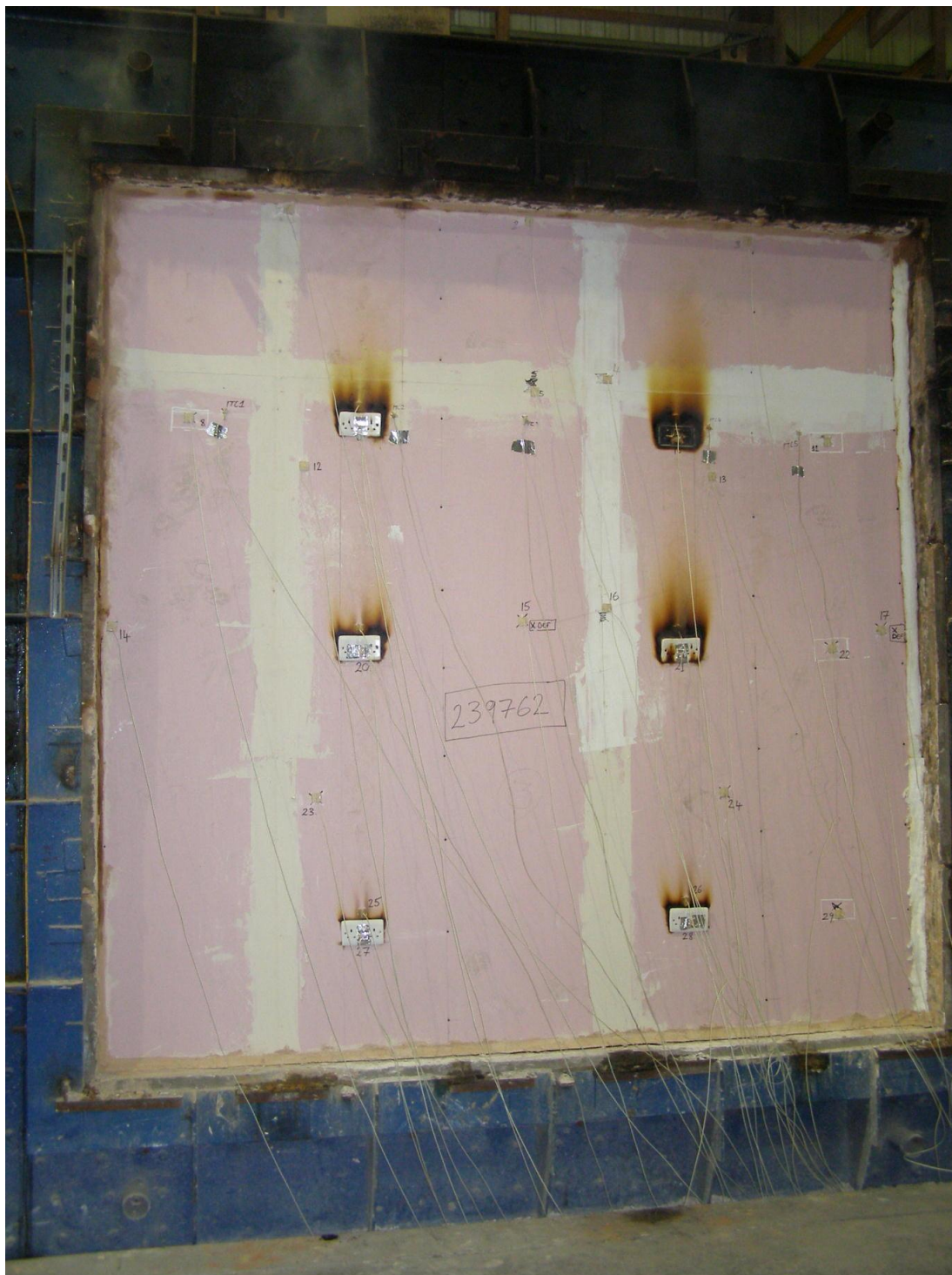
Photo 6: Unexposed face at termination of test, after 99 minutes duration
