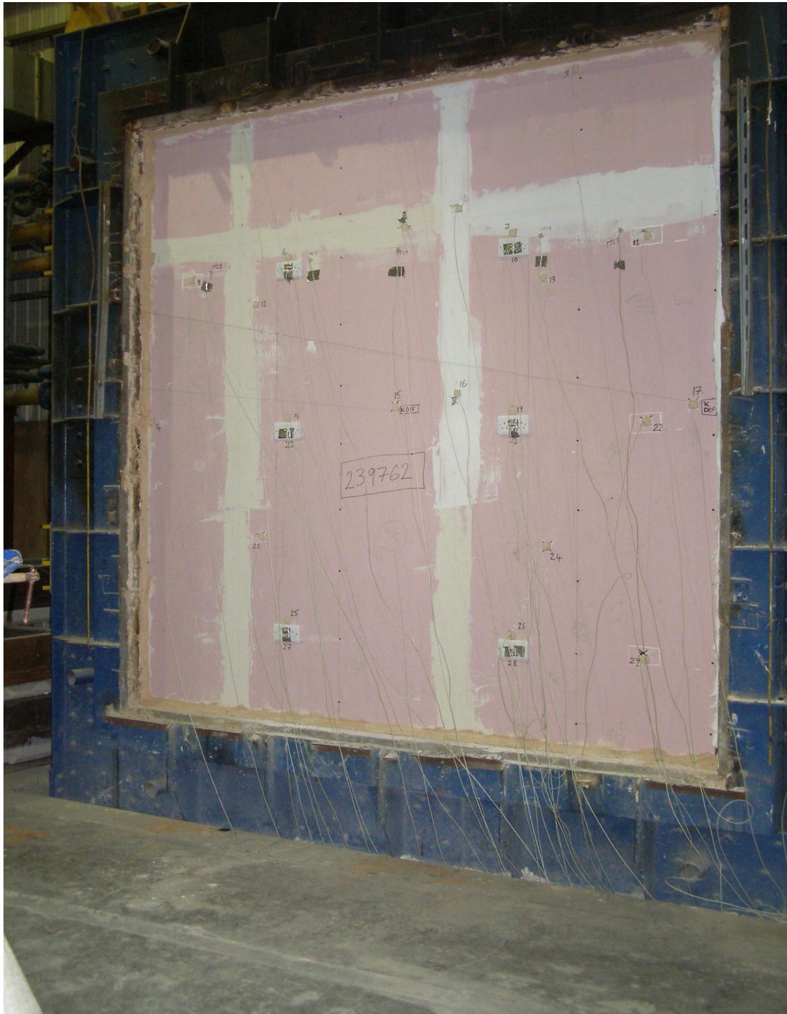
Photo 2: Unexposed face of the wall prior to start of test showing electrical sockets – from left to right - S2 and S3 (top row), S6 and S7 (middle row), S10 and S11 (bottom row)
