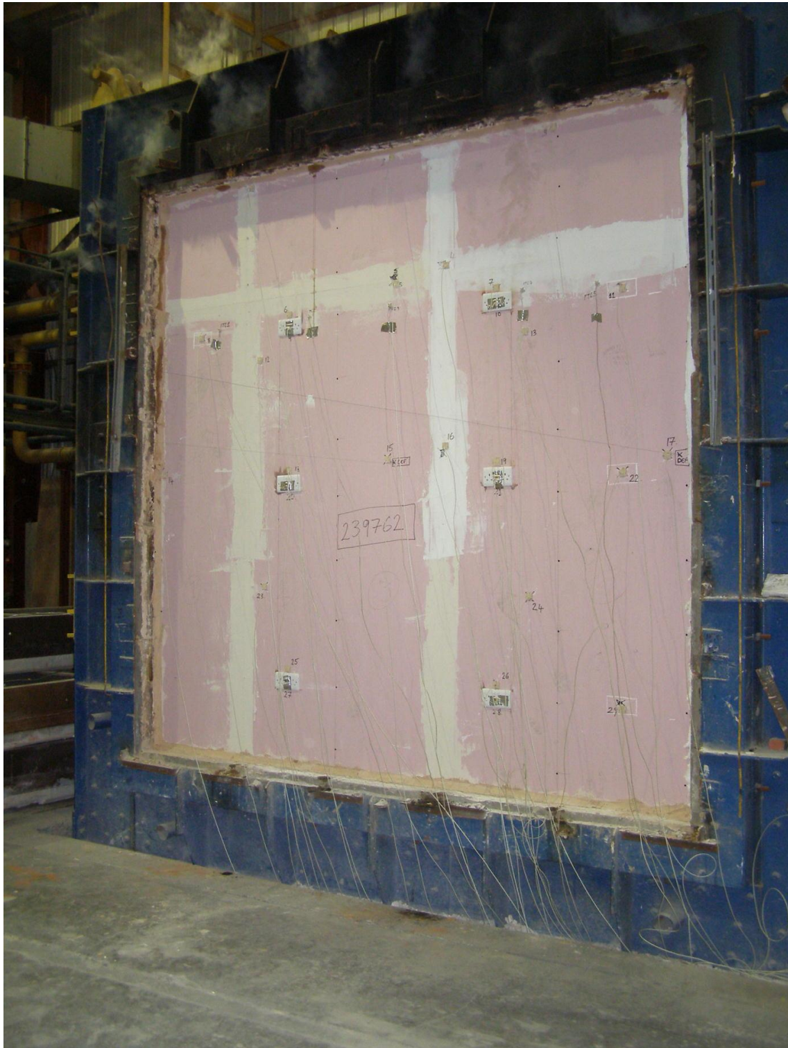
Photo 3: Unexposed face after 30 minutes from start of test
