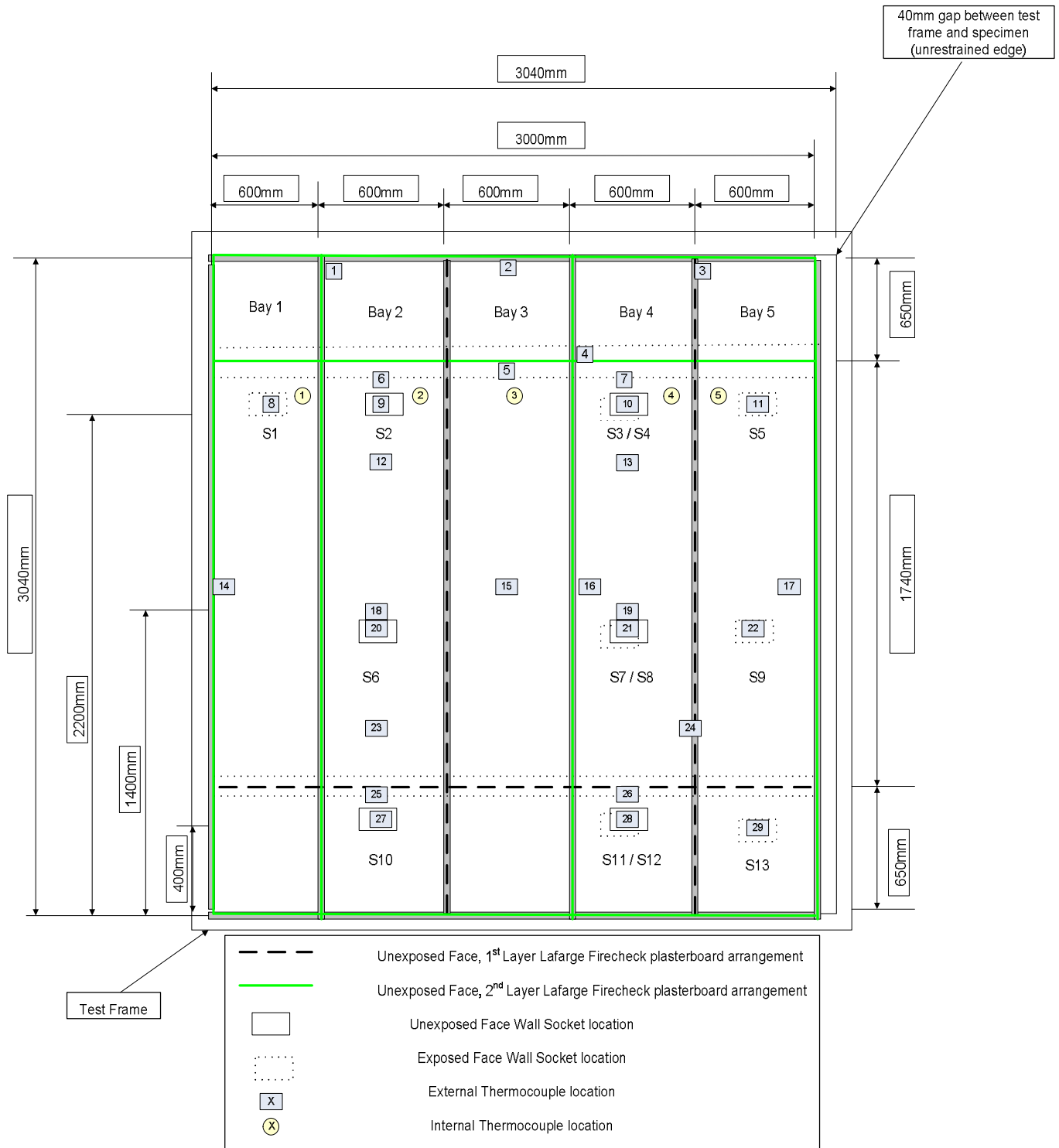
Figure 7: Showing the Internal and External Thermocouple locations on the Unexposed Face. (Drawing Not to Scale)
