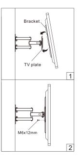
Tighten or loosen the M6 screws on the TV plate to keep it level Tighten or loosen the M8 screws on the TV plate
