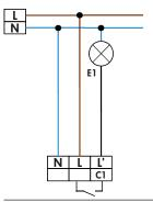
Standard mode with 1-channel motion detector with permanent light function
