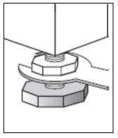
Once levelled correctly, you should tighten the lock nut back up on each of the washing machine feet using a spanner.
