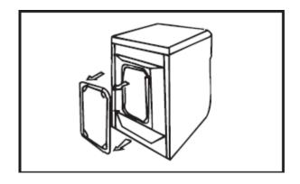
Remove the back plate from the rear of the appliance.
