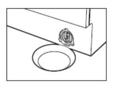
Place a container under the drain pump filter, to collect any excess water that may come out of the drain pump when it is removed.
