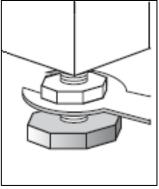
✓ Slacken off the lock nut on each of the washing machine feet using a spanner.
