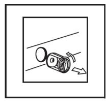
When all the water has drained out of the washing machine, turn the filter several times anti clockwise, until it can be removed completely.
