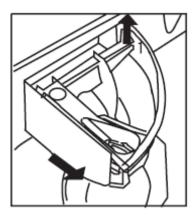
Swing open the detergent drawer and then remove the drawer by pulling it forward.
