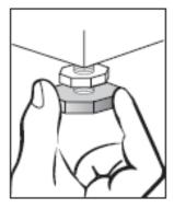
Adjust the feet to level off the washing machine.
