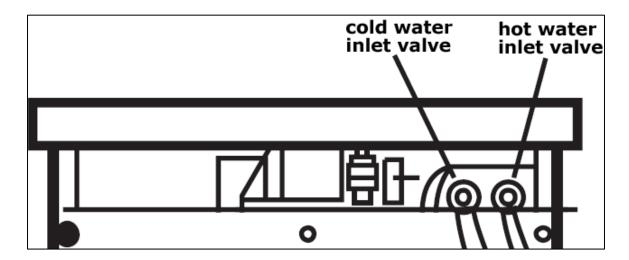
o When you are facing the **rear** of the appliance, you will see two water inlet valves next to each other. The cold water inlet valve is on the left hand side and the hot water inlet valve is on the right hand side.
