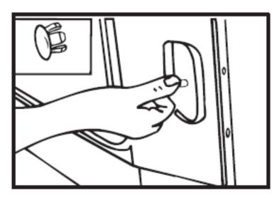
Insert the plastic caps that are supplied, into the holes that you have removed the transit bolts from.
