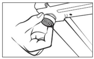
✓ Loosen the adjustable feet that are positioned on the base of the appliance.
