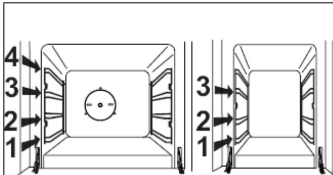
The oven walls are fitted with various guide bars on which you can place an oven shelf or a drip tray (see image below).
