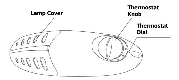
Your Fridge-Freezer's thermostat automatically regulates the inside temperature of the compartments. By rotating the knob from a lower to a higher numbered position, colder temperatures can be obtained. This is particularly important for food stored in the freezer.
