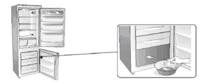
To accelerate the defrosting process, you can scrape off any frost that may have formed using the spatula included.
