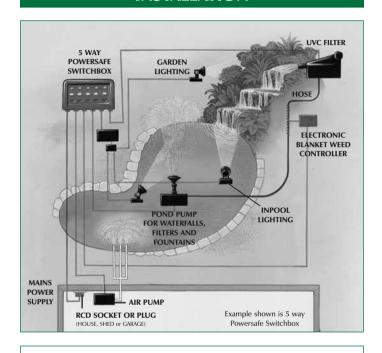
**IMPORTANT:** This outlet box is intended to be used with either a weatherproof cable connector or permanently connected to the fixed wiring of the mains system other than by means of a plug and socket. A Residual Current Device (RCD), also known as Residual Current Circuit Breaker (RCCB), having a tripping current not exceeding 30mA must be installed in the supply circuit.
