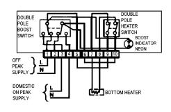
Wiring diagram for Hot water cylinders with single immersion heater.
