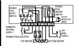
Wiring diagram for Hot water cylinders with dual or twin immersion heater.
