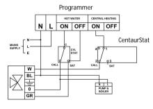
Horstmann CentaurStat replacing a conventional room thermostat on a fully pumped system with an existing programmer and 3 port mid-position valve.
