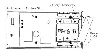
Once batteries have been fitted, offer the left hand side of the unit up to the mounting plate ensuring that the two guide lugs are fitted into the corresponding slots in the side of the mounting plate. Now swing the right hand side of the CentaurStat up against the mounting plate until the release button clicks into place.
