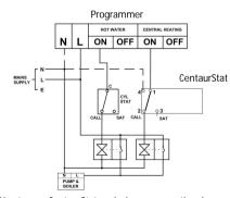
Horstmann CentaurStat replacing a conventional room thermostat on a fully pumped system with an existing programmer and two spring return valves with auxiliary switches.
