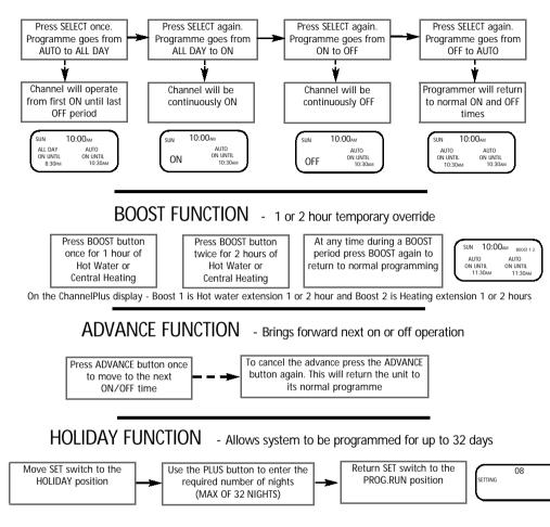
Whilst the HOLIDAY FUNCTION is in operation the system will remain OFF, the display will show the number of nights remaining. The HOLIDAY setting is an instant function and cannot be set in advance. The HOLIDAY FUNCTION can be cancelled at any time by pressing any of the SELECT buttons. Normal programme functions will resume at the first ON period after the pre-set number of nights has expired.
