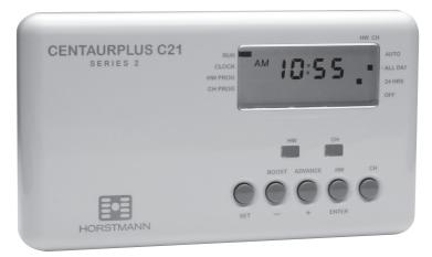
The Horstmann CentaurPlus C21 two channel programmer gives independent control over hot water and heating with up to 3 ON/OFF settings per 24 hours. It also has a 1 hour manual boost button for the hot water and an advance button for the central heating.
