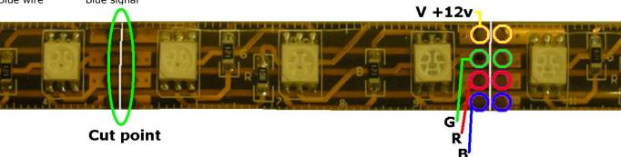
Each individual LED on the tape has three colour diodes mounted inside. They are the primary colours of Red, Green and Blue. When set at different intensities the light mixes and can produce many different colours
