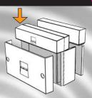
Remove two screws and unplug front panel of Telecom Master Socket. Plug the adaptor Faceplate in and replace front panel.
