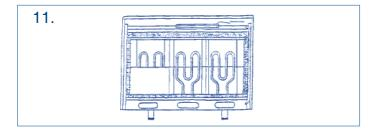
12. Fit the front layer of bricks again with the recess towards the element. The complete core will comprise:
