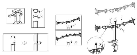
**Step 2** – Fit the desktop mount onto the table, the desktop depth should be between 15mm to 55mm. When fitting ensure the edge of the desktop is fully pushed in against the side of the clamp, also ensure the area clamped is as big as possible to allow load spread. Fully tighten the clamp when desktop is in place.
