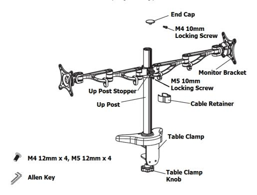
For this installation you will also require a tape measure and a Philips (cross) screw driver.
