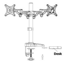
**Step 3** – Mounting screens. After checking the desktop mount is installed firmly, the monitors can now be installed on to the mount. Check the weight of each monitor is no more than 8kg before installing. Use the correct sized screws for your screen from the screws supplied and fit the screen on as shown in the diagram below. Tuck all cables into the cable management hook at the bottom of the bracket to finish the installation.
