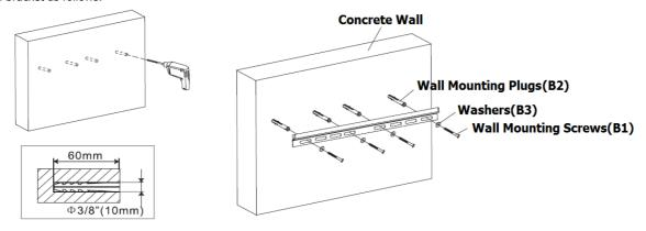
For plaster wall installation first of all find out where the wood stud is behind the wall using a stud finder. Then work out the height of the installation and ensure it is level using the spirit level. Use a pencil to mark where the mounting holes will be and use an electric drill to drill a hole that is around 5mm in diameter and 60mm deep. Install the wall bracket as follows.
