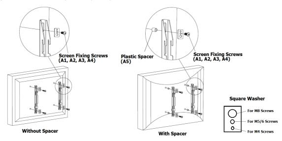
Step 3 – Hook the TV bracket on to the wall mount and gently rest the TV against the wall as shown below.
