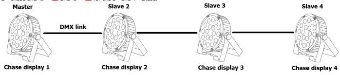
More units can be arrayed together to work as a group such as below to perform the same light display or sequential chase. Each group will display the same output in sync with the master unit:
