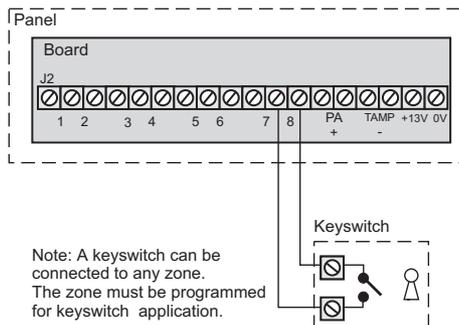
The keyswitch may be used to Set (open contacts) or Unset (closed contacts) independently of RKPs. However in this situation the keyswitch may have to 'catch up' with the system. For example if the system is Set via an RKP and Unset with the keyswitch, it
