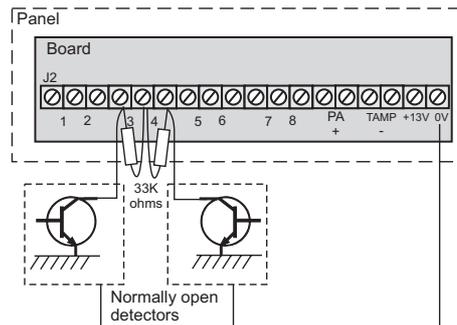
The example below shows how to wire normally open detector on zones 3 and a normally closed detector on zone 4.
