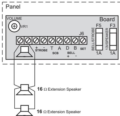
Up to two 16 ohm extension speakers may also be wired across the speaker terminals. Mounted in convenient positions within the installation the extension speakers will reproduce all of the alarm tones generated by the control panel.
