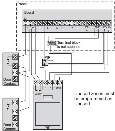
**Note:** The G3 range of panels are **not supplied with wire links** for unused zones. All unused zones must be programmed out by setting them to *disabled* using the **Zone Type** function see page 19.
