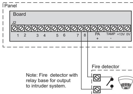
There are two types of fire zone, **Standard** and **24 hour** type. The **Standard fire** zone detects fires only when the system is Set, whereas the **24 hour fire** zone detects fires all the time and will operate whether the system is Set or Unset. A fire will cause a distinctive internal sounder tone. The external sounders will pulse on and off at 2 second intervals and all RKP indicators will flash the affected zone.
