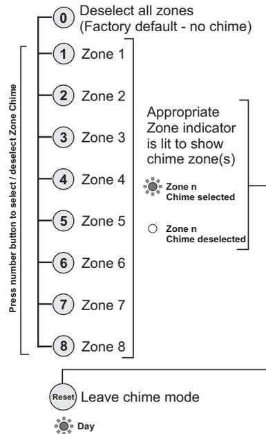
Chime is a low security monitoring system for use when the system is Unset. When a zone that is set to chime is operated, the internal sounder will produce a low volume two stage warning tone and the Zone indicator will show. The indicator may be cancelled by pressing Reset. Chime is particularly useful in a shop to warn of a customer presence or in a house to warn that a door or particular area has been accessed.
