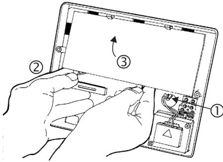
**Note:** When replacing the PCB align it on the round support pillars to the bottom and allow it to click down past the clips at the top of the case. Refit the transformer wires into the terminal.
