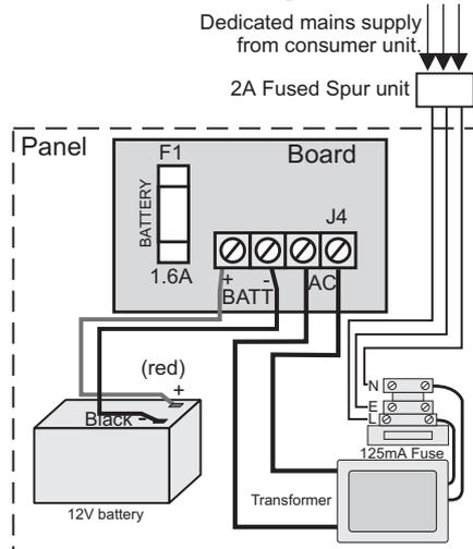
**Note:** The mains supply must be connected by a technically competent person and according to current IEE regulations.
