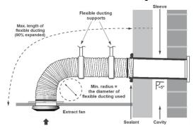
Where flexible ducting is used the diameter must be maintained and it is good ventilation practice that the ducting is extended to a minimum of 90% its possible length in order to maintain the best possible air flow.
