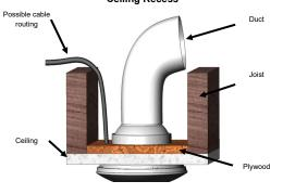
The fan should be fitted in the hole, fixed with the screws provided into the support.
