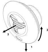
To refit the cover, reverse the above procedure. If when refitting the front cover the iris stays open, remove the cover and don't attempt to refit it for approx. two minutes (allowing the actuator to retract back in the closed position). Then try again.
