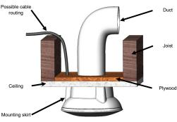
When surface mounting the iCON 30 and iCON 60, the mounting skirt provided should be used. The mounting skirt should be fixed, with the screws provided, into the support. The fan is then fitted into the skirt.
