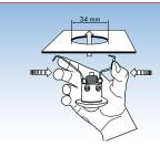
Make a circular opening of diameter max. 34 mm into the ceiling. Having connected up the cables in accordance with regulations, the occupancy detector to be connected to the power supply by means of the RJ11 plug and the detector is inserted into the opening as shown below and fixed into position with the assistance of the spring clips.
