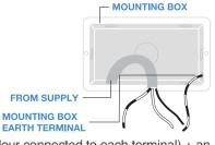
be two or three wires of each colour connected to each terminal) + an additional connection between the mounting box earth terminal and the socket earth terminal.
