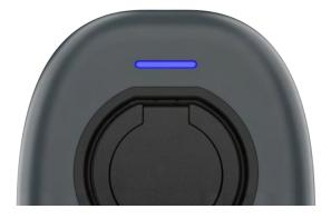
In less than 2 minutes, the indicator should turn from Yellow to Blue to confirm network connection.
