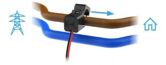
Open the CT Clamp and fit around the incoming Live power cable, this is typically marked brown for most installations.
