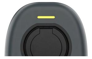
Upon powering the charger, the status indicator light will show Yellow. This indicates that the charger is ready for network setup but is not yet connected to the internet.
