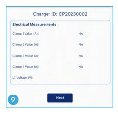
Check the shown electrical measurements match measured readings. This will allow checking the Load management CTs are fitted correct orientation.
