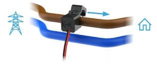
Open the CT Clamp and fit around the incoming Live power cable, this is typically marked brown for most installations.
