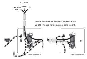
All earth wires must be sleeved and terminated to the back box
