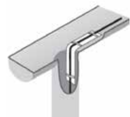
GP-S spacer protecting GP-18 cable from a sharp edge
