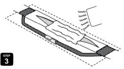
Now slide the 150mm length of heat shrink over the entire joint area and, again using the heat gun, shrink into position. The splice is now complete.
