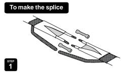
Using the 2 blue insulated barrel connectors' crimp the Buss conductors together red to red and blue to blue.
