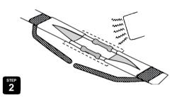
Slide the 70mm heat shrink so that it is centred over the joint and shrink into position. Using the uninsulated barrel connector, butt the earth 'pigtails' into the connector and crimp.
