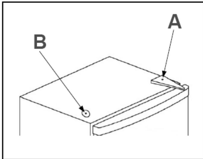
7) Carefully slide the upper door from the upper hinge pin (**K**) and then using a star head screwdriver unscrew the top hinge cover (**A**) and sensor cover (**B**).
