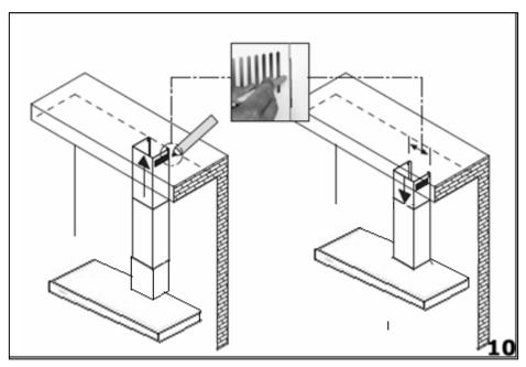
**10)** Lift chimney section **D** upwards until it reaches the ceiling. You must ensure that it is perpendicular to the hood.
