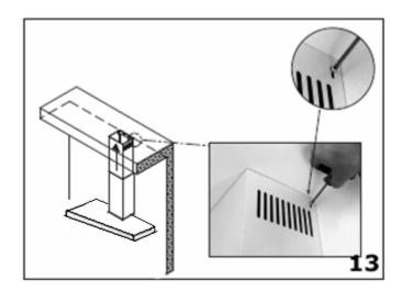
Slide chimney section **D** inside of chimney section **C**. Then secure the upper bracket to the wall, using the same method as you have just used to secure the lower bracket.
