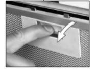
**1)** Remove the metal grease filters.
