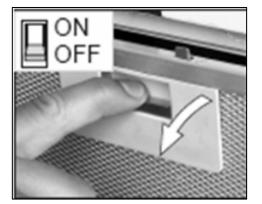
First remove the grease filter by pulling down on the handle, and then pull it upwards away from the main body of the cooker hood.
