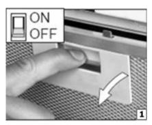
1) Remove the grease filters.
