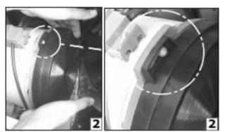
2) Hook the carbon filter over the pins that are located at the end of the motor.
