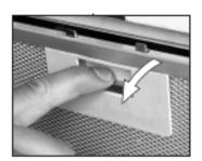
**1)** Remove the metal grease filters.
