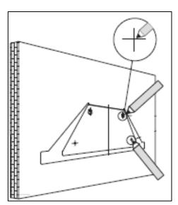
2) Position the hood against the wall that you are intending to install it on and mark the position of the support holes that are to be drilled (as shown in the figure opposite).
