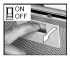
o Refit the grease filter.
