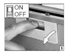
1) Remove the grease filters.
