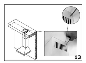
${f 13}$ ) Lift chimney section  ${f D}$  up to the ceiling and secure it to the fixing bracket using the screws provided.
