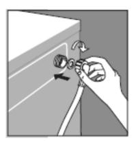
✓ Connect and fully tighten the inlet hose to the threaded inlet valve that is located at the rear of the washing machine. You should connect the end with the right angle connector on it to the back of your appliance.
