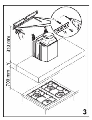
**3)** Measure a distance of 700 mm from the hob top that will be underneath the cooker hood. Then measure out a further 310 mm above the height of measurement Y (Y being the thickness of the canopy section of the cooker hood).
