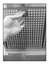
1) Remove the metal grease filters.
