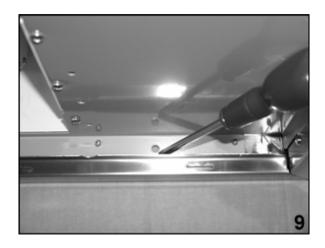
9) Mark the position of the lower screw holes that need to be drilled out in step 10. The holes can be found immediately below the motor housing. (The position of one of the holes is indicated in the above photograph by the screwdriver).
