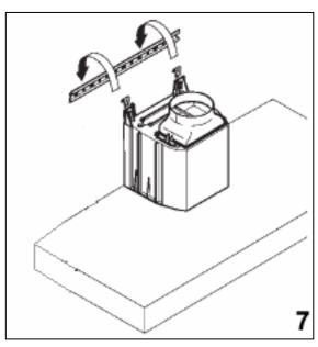
**7)** Hook the hood onto the mounting bar.
