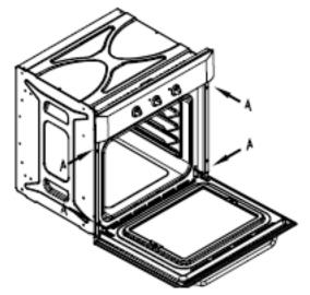
Ensure that the oven has been securely fixed into the housing unit. The fixing of the oven into the housing is made by using four screws. These should be screwed through the oven cabinet and into the housing unit.
