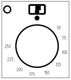
The oven thermostat control knob sets the required temperature of the oven. It is possible to regulate the temperature within a range of 50 - 250°C.
