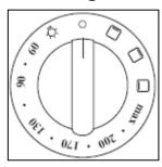
If you turn the control knob clockwise, it will automatically select the oven light function first. If you continue turning the control knob, you will select the conventional oven function. You can regulate the conventional oven between a temperature of 50 - 250°C.
