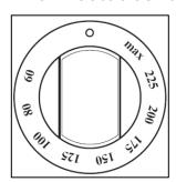
The oven thermostat control knob should be turned clockwise and it sets the required temperature of the oven. It is possible to regulate the temperature within a range of 50 - 250°C.
