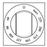
o Use this control knob to control the temperature in the oven.
