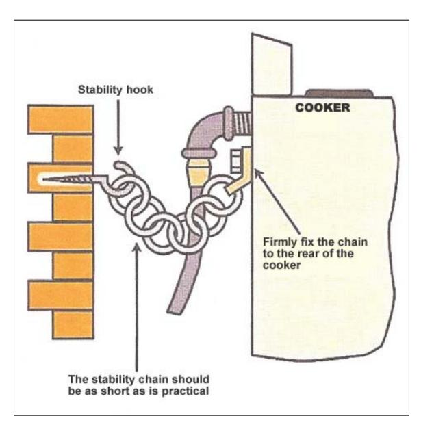
The stability hook should be securely fixed to the fabric of the building, in an adjacent position to the safety chain at the rear of the appliance.
