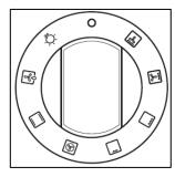
Use this control knob to select the oven function and turn on the oven light in the main oven.
