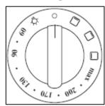
If you turn the control knob clockwise, it will automatically select the oven light function first. If you continue turning the control knob, you will select the conventional oven function. You can regulate the conventional oven between a temperature of 60 - 250°C.
