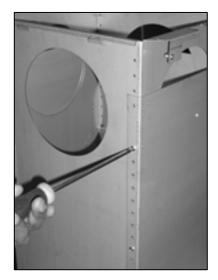
**8b)** To make an adjustment to the height of the framework, unscrew the 8 screws that hold it in place, lift the framework to your required height and refix the 8 screws into the framework.
