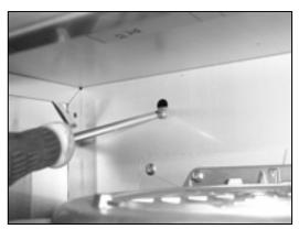
**3)** From inside of the motor housing, undo the four screws that hold the framework in position.
