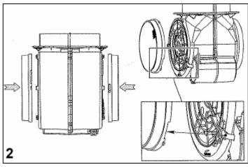
2) Place a carbon filter at both sides of the motor. You should make sure that the cut out in the rim of the carbon filter, lines up with the lug on the motor.
