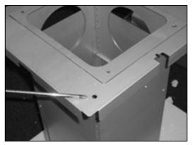
**12)** To reinforce the upper plate, you should drill into the ceiling, through the holes on each corner of the upper plate. The position of one of these screw holes is shown in the photograph. You should use an 8 mm diametre drill bit.
