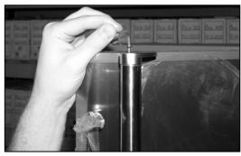
6) Use the allen key supplied to fully tighten the screws at the top and bottom of the handle.
