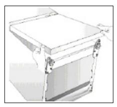
5) Remove the lower door by gently sliding it downwards, away from the main body of the fridge freezer.
