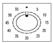
The minute minder can be used independently of an oven cooking function for a time period of up to 60 minutes.
