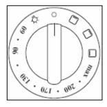
If you turn the control knob clockwise, it will automatically select a conventional oven function and you can regulate the temperature between 60 - 250°C.
