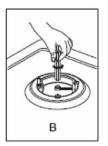
Unscrew the injector (B) and replace it with the stipulated injector for the new gas supply (see table below).
