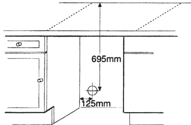
If the through the wall vent is to be positioned other than behind the dryer, the vent hose should be positioned at floor level and through adjacent side panel to a relevant position.
