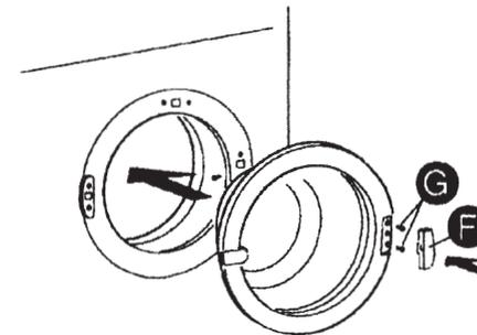
3. Reverse the door and place against the dryer's doorway so that it is in the closed position. Refit the screws (G) and hinge cover (F). Open the door.
