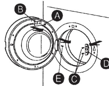
1. Open the door. Undo the screw (A), remove the switch strike (B) and replace the screw. Remove the screws (C) and latch plate (D). Remove the hinge cover screw (E). Close the door.
