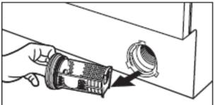
When all the water has drained out of the washing machine, turn the filter several times anti clockwise, until it can be removed completely.
