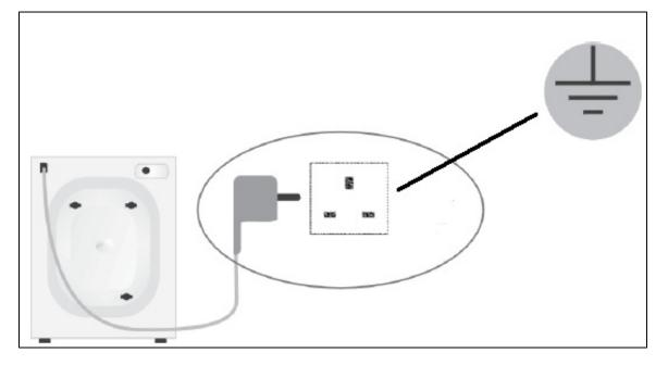
✓ IMPORTANT: The electrical socket must still be accessible once the appliance is installed.
