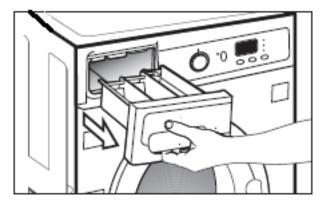
Pull the detergent drawer out as far as it will go and then remove the drawer by pulling firmly.
