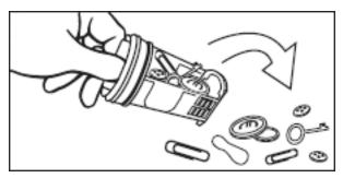
Remove the filter and rinse out the filter under the tap.
