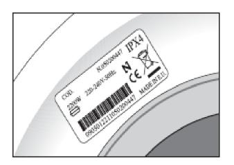
Consult the rating plate, located on the inner rim of the porthole door of the appliance **BEFORE** making the electrical connections. Ensure that the voltage reaching the plug, is the same as that on the rating plate.
