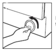
Remove the kickplate and then use a coin to turn the filter cap.
