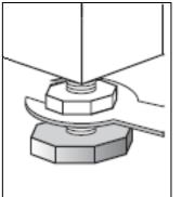
✓ Slacken off the lock nut on each of the washing machine feet using a spanner.
