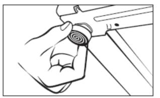
✓ Loosen the adjustable feet that are positioned on the base of the appliance.
