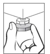
Adjust the feet to level off the washing machine.
