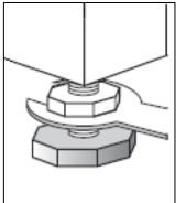
✓ Once leveled correctly, you should tighten the lock nut back up on each of the washing machine feet using a spanner.
