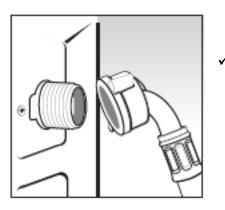
✓ Connect and fully tighten the inlet hose to the threaded inlet valve that is located at the rear of the washing machine. You should connect the end with the right angle connector on it to the back of your appliance.
