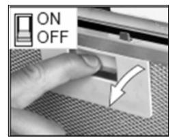
First remove the grease filters by pulling down on the handle, and then pull it upwards away from the main body of the cooker hood.
