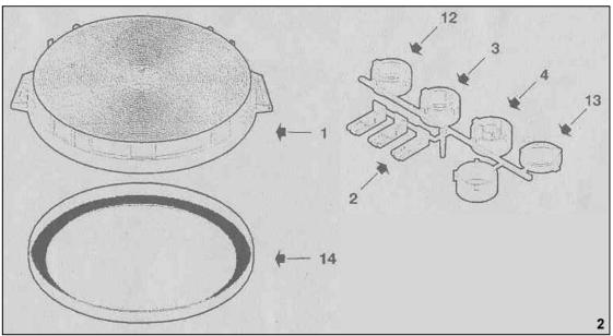
2) The UCF1 carbon filter is a universal filter; you do not require all of the parts that are supplied with it. For the CAN54SS you will require parts 1 and 13.
