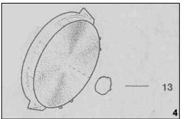
4) Insert part 13 into part 1 of the carbon filter.
