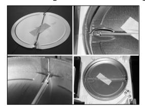
You may find an anti-draft flap included with the fixtures and fittings for the cooker hood. If you are going to duct the product externally, you should fit this as shown in the circular hole on top of the motor.
