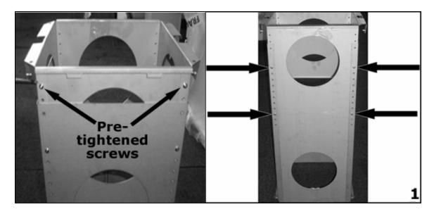
1) If you are installing the product at minimum height, then you need to remove the 10 screws from the framework, including the 2 pre-tightened screws. Separate the inner and outer sections of the framework.
