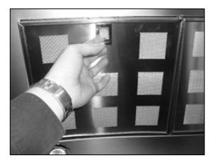
Remove the grease filters.
