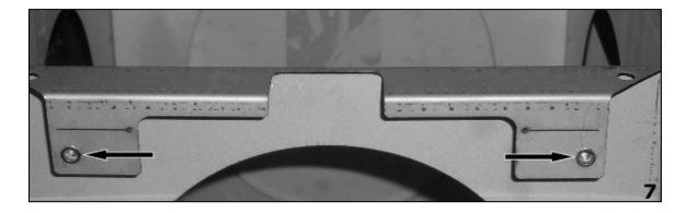
**7)** Lift the chimney section up to the framework and then fasten it to the framework using the 4 x M4 metric screws supplied. The chimney section should be fixed to the existing holes in the framework. **IMPORTANT:** Do not tighten these screws completely at this stage.
