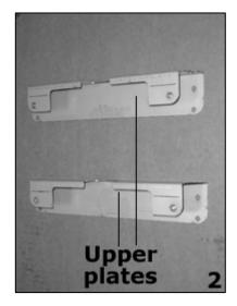
**2)** Remove the 4 rivets that hold the upper plates onto the inner framework.
