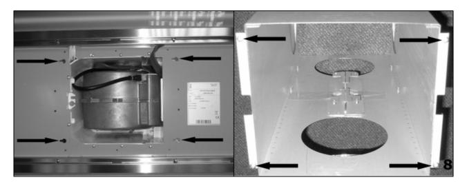
**8)** Raise the hood to the framework and locate the 4 M5 screws on the bottom of the framework into the 4 holes that are around the outside of the motor housing. Slide the hood over to the right so the hood locks against the framework and then fully tighten the 4 M5 screws.
