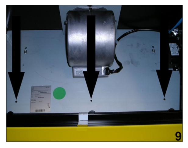
**9)** From the inside of the cooker hood, mark the position of the three lower screw holes that need to be drilled out.
