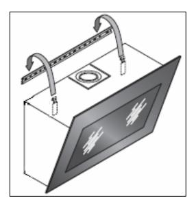
**7)** Hook the hood onto the mounting bar.
