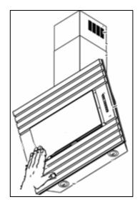
Open the cover screen at the front of the cooker hood, this will allow you to gain access to the grease filters.
