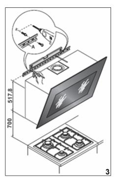
**3)** Measure a distance of 700 mm from the hob top that will be underneath the cooker hood. Then measure out a further 518 mm above this height.
