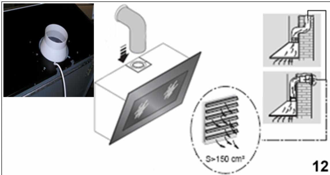
**12)** Connect the coupling to the top of the cooker hood, and then connect a 125 mm ducting hose to the coupling. Please note that the ducting hose is not supplied with the appliance. \*
