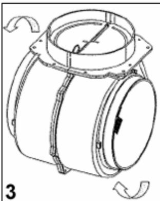
3) Turn the each of the carbon filters clockwise until they lock securely into place.
