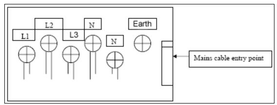
o The cable connections must be in accordance with the diagram located on the bottom of the hob.
