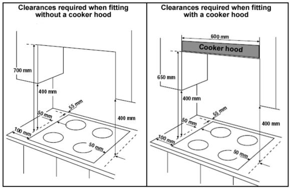
This appliance is classified as Class 3 and therefore is to be built into a kitchen unit (depending on size) or 600 mm worktop, providing the following minimum distances are allowed:
