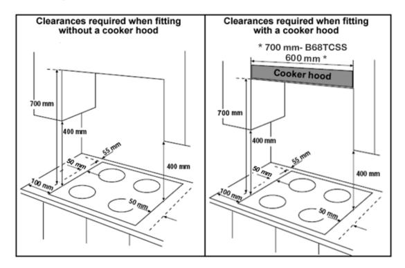
This appliance can be located in a kitchen, a kitchen diner or a bed sitting room. IMPORTANT: The appliance must not be installed in a bathroom or shower room.
