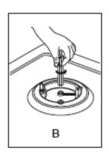
Unscrew the injector (B) and replace it with the stipulated injector for the new gas supply (see table below).
