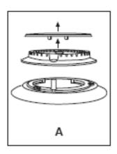
o Remove the pan-stands, burners and flame spreaders (A).
