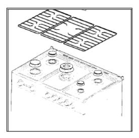
Remove the pan-stands, burners and flame spreaders.
