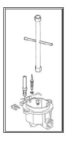
Unscrew the injector and replace it with the stipulated injector for the new gas supply (see table on next page).
